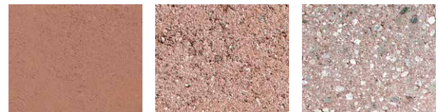
Smooth Shot Blast Ground Face
