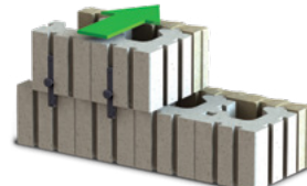
STEP 3 - Push the units forward until they lock
