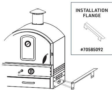
After your island is made with the correct cut out dimensions, and you have your flanges attached, slide your oven into your cut out. Then plug in your electrical and connect gas to your oven.
