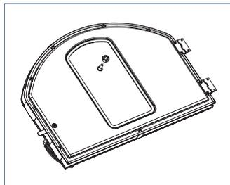
6. Use M4\*10 screw \* 4 pcs to fix the door onto the oven. Now you have finished cleaning the oven door.
