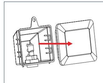
5. After replacement, use one hand to hold the metal back part of the light and one handle to hold the front glass cover and then clip them together in the right position.
