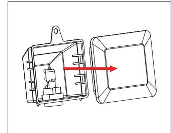
5. After replacement, use one hand to hold the metal back part of the light and one handle to hold the front glass cover and then clip them together in the right position.
