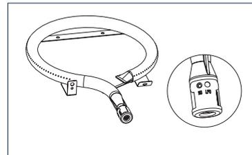
Use orifice removal tool to remove the 1.2 LP orifice from the oven. And then use the same tool to fix the 1.8 NG orifice back to the position.
