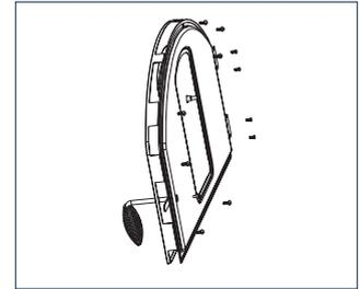
3. Use spanner 19# to loosen the nut that fix the temperature gauge. And then you can completely separate the oven door exterior and interior so as to do the cleaning.
