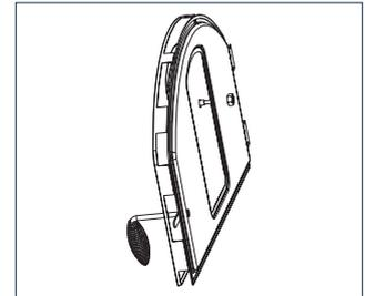
4. After cleaning, you need to re-assemble the oven door. Put the door interior onto the exterior and make every screw hole in line with each other. Use M4\*10 screw \* 7 pcs to fix the door interior and exterior. And then use shoulder screw to fix the handle onto the door. Finally, use M4\*10 screw \* 4 pcs to fix the hinge onto the door.
