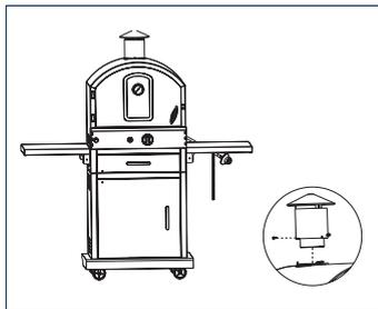
2. Use screw M5\*35×4 pcs to fix the back heat shield onto the back panel of the oven. The order is: screw, back heat shield, heat insulation washer, flat washer, oven back panel.
