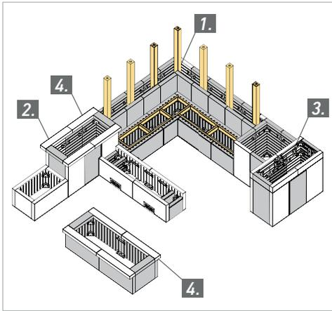
**1.** Drill the concrete panel to install the Concrete Screw Anchors, and the wood post to install the Stainless Steel Screw.
