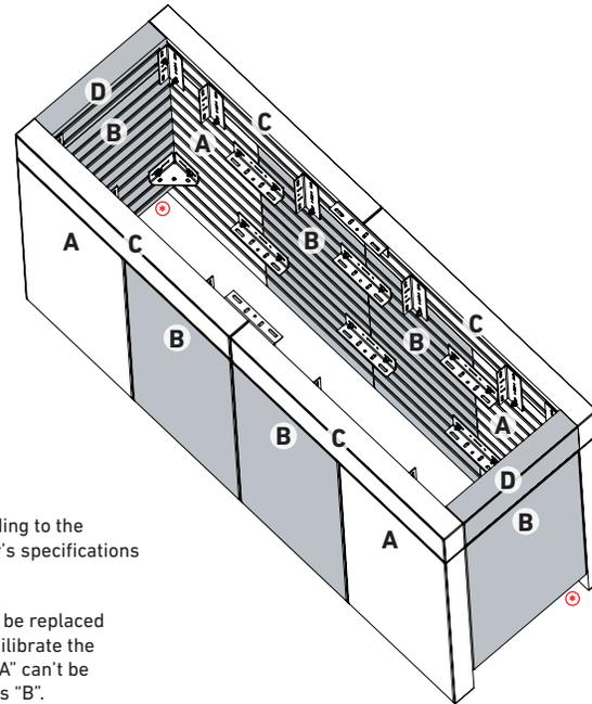
Ⓞ Cut panel(s) according to the burner manufacturer's specifications for ventilation.
