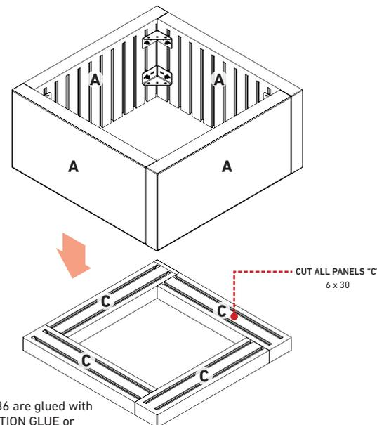
**NOTE:** The panels 18 x 36 are glued with 6 x 36 using CONSTRUCTION GLUE or STRUCTURE BOND
