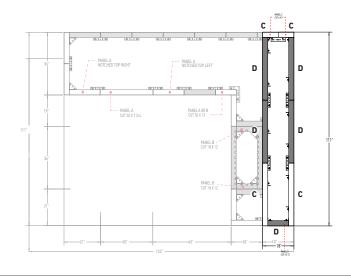
**REQUIRED PANELS** 18 x 36 PANEL 10x 18 x 36 PANEL 4x 5x IMPORTANT: 18 x 36 panels are sold in pair/layer or in full pallet only. 6 x 36 panels are sold per unit or in layer or in full pallet. **REQUIRED HARDWARE** ANCHOR SLIDE AND NUT 150x JOINING PLATE 22x OUTER CORNER 6 x 0 x STRETCHER TOTAL WEIGHT 5105 Lbs
