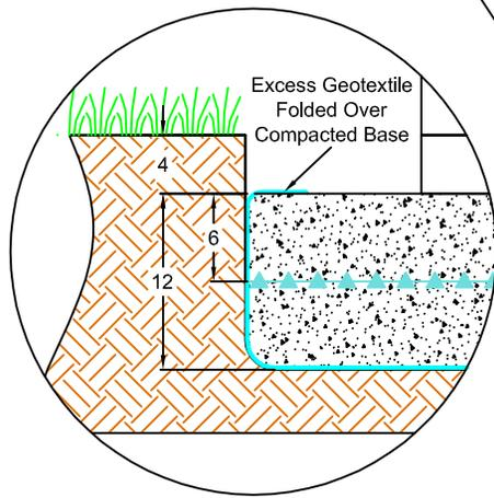
$\frac{3}{4}$ " minus Road Base Material, Compacted in 2 to 3 inch lifts (lightly hydrated during compaction, but not saturated).
